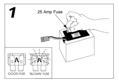
• If you are charging the battery for the first time, insert a 25 amp fuse into the battery.
